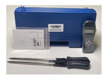
MC-7825G grain moisture meter used for fast and accurate measurement of moisture in the process of allotment, acquisition, storage, machining of packed grains, feedstuff, powder.
